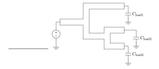
We divide the wires into 6 segments of fixed length  $l_i$ ; our variables will be the widths  $w_i$  of the segments. (The height of the wires is related to the particular IC technology process, and is fixed.) The total area used by the wires is, of course,
