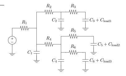
We will use the Elmore delay to model the delay from the source to each of the loads. The Elmore delay to loads 1, 2, and 3 are given by
